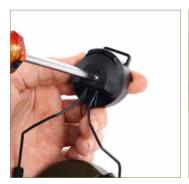
1. Unmount device from helmet. Disassemble mount by unscrewing phillips head screw. Remove rear plastic portion.
